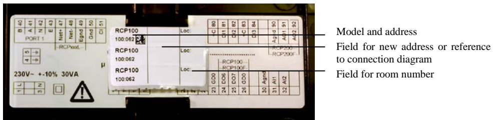
Figure 1. Label on the back of the RCP-controller
