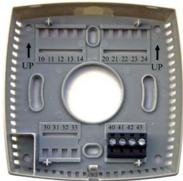
Figure 7. RU bottom plate with location of terminals
